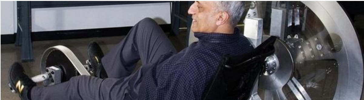
Manoj Bhargav created Free Electric, a stationary cycle that can light up 24 bulbs, run an electric fan, and charge a cell phone and a tablet when pedaled for an hour.
